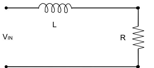
$$\frac{V_{OUT}}{V_{IN}} = \frac{R}{R + j\omega L}$$
