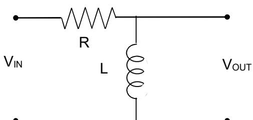
$$\frac{V_{OUT}}{V_{IN}} = \frac{j\omega L}{R + j\omega L}$$
