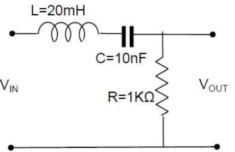
$$A) \frac{V_{OUT}}{V_{IN}} = \frac{R}{R + j\omega L + \frac{1}{j\omega C}} = \frac{j\omega RC}{1 + j\omega RC + j^2\omega^2 LC} = \frac{j\omega RC}{(1 - \omega^2 LC) + j\omega RC}$$
