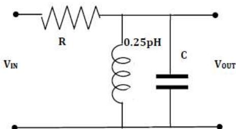
$$G(\omega) = |H(\omega)| = \frac{\frac{1}{\omega RC}}{\sqrt{\left(\frac{1}{LC} - \omega^2\right)^2 + \left(\omega \frac{1}{RC}\right)^2}}$$
