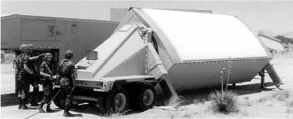
FIGURE 1-42 ■ Photograph of the Terminal High Altitude Air Defense AN/TPY-2 radar. (Courtesy of U.S. Missile Defense Agency.)
