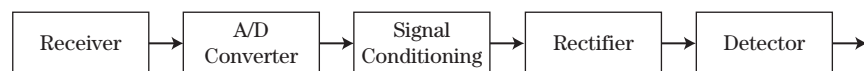
FIGURE 16-1 ■ In a modern radar, the processing chain operates on digital data to maximize SINR, detect targets, and control false alarms.
