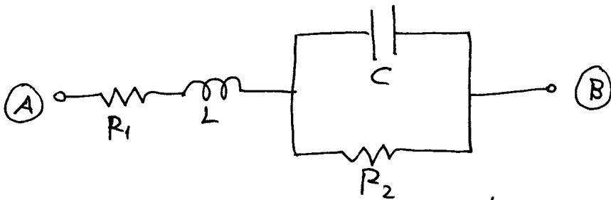
$$Z_{AB}(D) = R_1 + LD + \frac{R_2 \frac{1}{CD}}{R_2 + \frac{1}{CD}}$$
