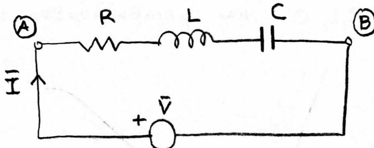
$$\text{ii} \quad \bar{Z}_{AB} = R + jX = R + j\omega L - \frac{j}{\omega C} = R + j\left(\omega L - \frac{1}{\omega C}\right)$$
