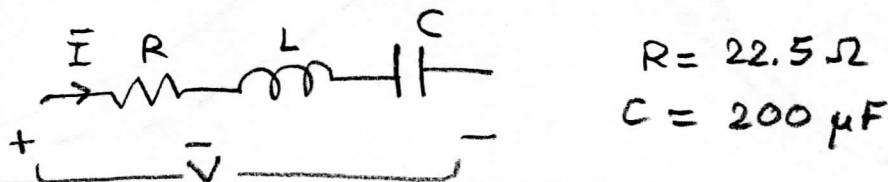
$$\text{Έχουμε: } \bar{Z}(\omega) = R + j\left(\omega L - \frac{1}{\omega C}\right) = |\bar{Z}(\omega)| e^{j\varphi_Z(\omega)}$$
