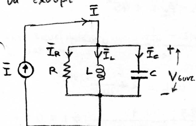
$$\bar{I}_L = \frac{\bar{V}_{6\text{vurz}}}{j\omega_{6\text{vurz}} L} \quad (\text{όπου } \bar{V}_{6\text{vurz}} = \bar{I} \cdot R)$$
