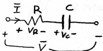
$$Q = 2\pi \cdot \frac{\frac{1}{2} C V_{cm}^2}{\frac{1}{2} I_m^2 R T} = 2\pi \cdot \frac{C V_{cm}^2}{(V_{cm}/\omega C)^2 R T} \Rightarrow$$
