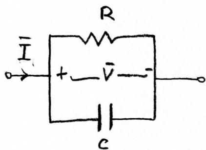
$$Q = 2\pi \cdot \frac{\frac{1}{2} C V_m^2}{\frac{1}{2} I_m^2 R T} = \frac{2\pi \cdot C V_m^2}{(\frac{V_m}{R})^2 R \cdot \frac{2\pi}{\omega}}$$
