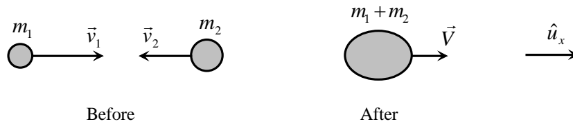
Fig. 6.6 Plastic collision of two masses.
