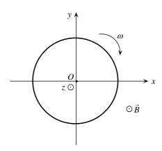
Both the *z*-axis and the magnetic field are normal to the page and directed toward the reader; the direction of motion is clockwise (why?).
